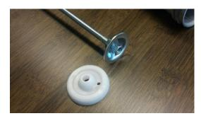
2) The metal flange is held in place by the screws. Unscrew the first one and place it inside the white flange. You can now screw the flange back onto the threaded rod. The second screw at the back is to position the flange and to tighten it onto the rod.
