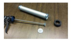
1) Disassemble the silicone sausage foil gun.
